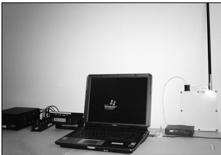
Figure 6 — The components of the integrated network are pictured left to right: Astron power supply, MFJ power strip, Yaesu FT-8800 transceiver with KPC3+ TNC sitting on top, Winbook laptop with Paclink AGW, Paclink Post Office and AGW Packet Engine software installed. To the right of the server is the SMC router and behind the router is the DWL-2100AP modified by NETKROM.
