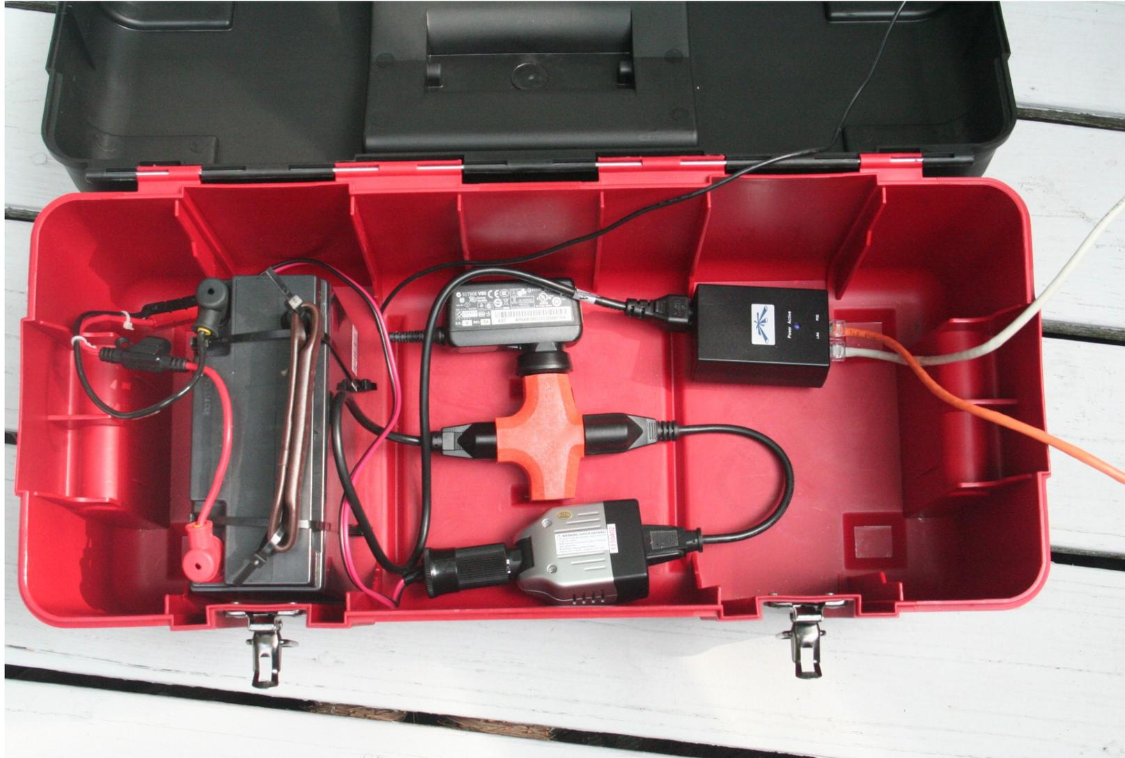
18 aH battery, 75 W power inverter, Ubiquiti 48 V POE adapter
