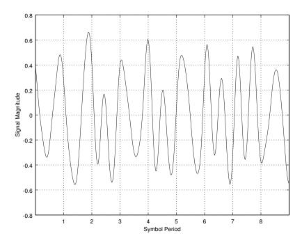
Figure 2: Amateur Bell 202 signal representing the ASCII letter A (0x41)
