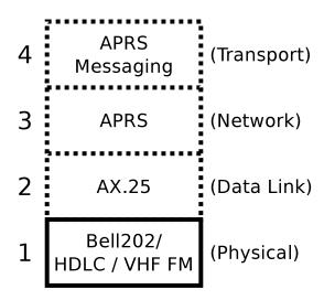
Figure 1: OSI network layers for a typical packet radio application. This paper refers to the entirety of layer 1 as "Amateur Bell 202"
