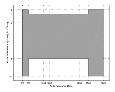
Figure 6: Allowable distortion in a basic 3002 telephone channel
