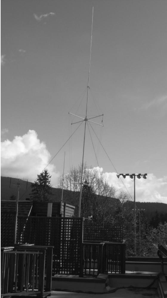
Big antennas are not only more efficient and sensitive they are also a lot less interference prone due to local near field changes. This means that some maintenance can be done without having to turn off the RF-Seismograph. Especially when the monitoring is done over long periods of time, maintaining the antenna, while recording, with a minimum of interference, is a big plus.
