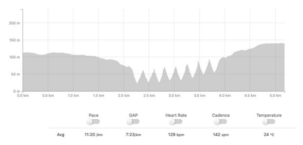
These types of problems are generally corrected by calibrating the pressure sensor using GPS altitude as well as other information sources. As can be seen here, this is not always successful.
