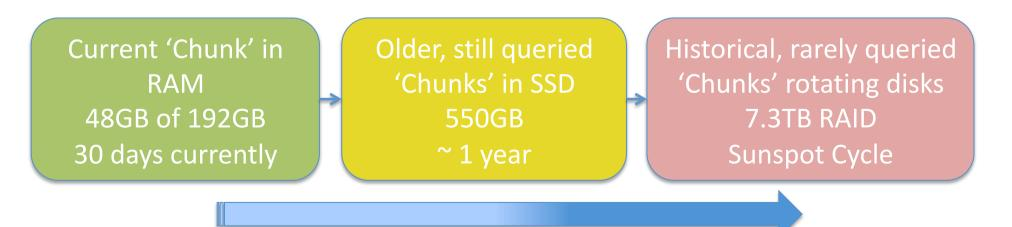
Data movement over time to higher capacity, less expensive storage
