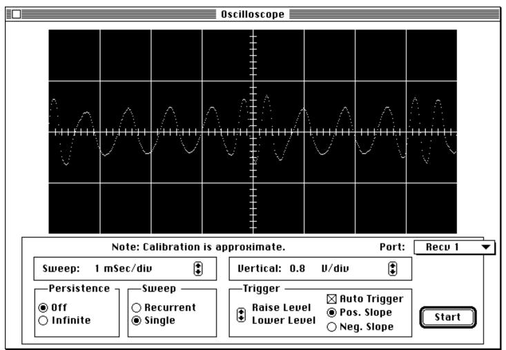
Oscilloscope: The display shows a 1200 bps packet audio signal. Note the two different periods of the waveform corresponding to different binary digits.
