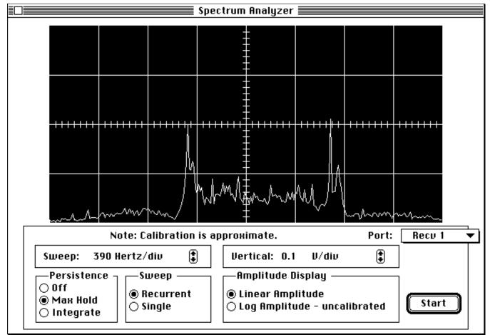
Spectrum Analyzer: The display shows a 1200 bps packet audio signal. Note the two peaks corresponding to the low and high tones of the AFSK signal.
