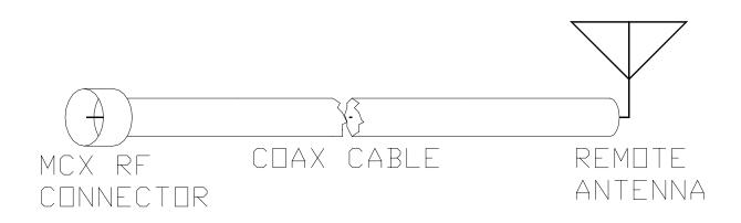
The recommended GARMIN remote antenna for the GPS 25LP series is the GA27. It has eight feet of RG-174A/U type cable with a MCX connector installed for attachment to the sensor board. An extension cable with up to -5dB additional attenuation at 1.5 GHz may be used with the GA27 (either 50 Ohm or 75 Ohm impedance cable is permitted).
