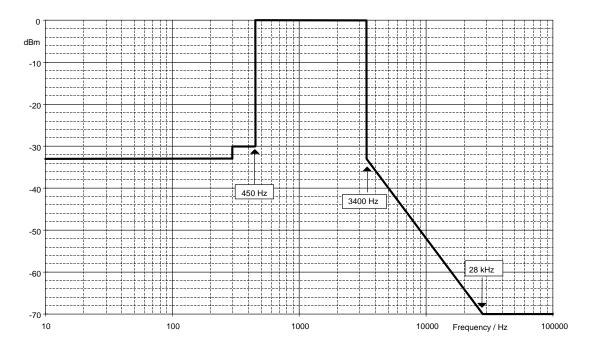
Figure 6: Tx limits at 1200bps rate
