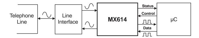
The MX614 is a low voltage, low power CMOS integrated circuit designed for the reception or transmission of asynchronous 1200bps data. This device is compatible with Bell 202 type systems. The MX614 supports 5bps and 150bps 'back channel' operation.
