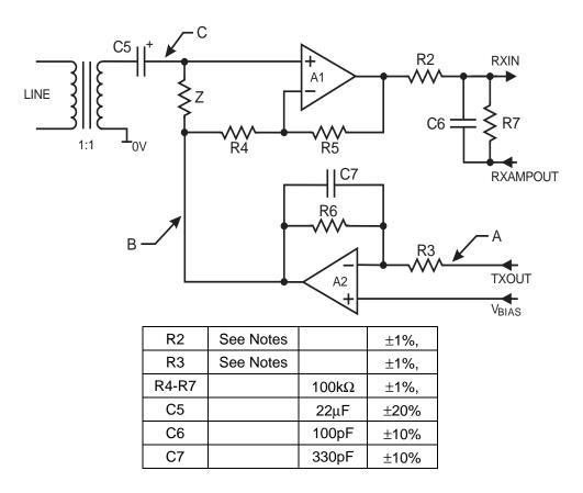
Figure 11: Line Interface Circuit
