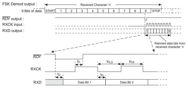
$t_D$  = Internal MX614 delay,  $t_{CHI}$  = CLK high time,  $t_{CLO}$  = CLK low time
