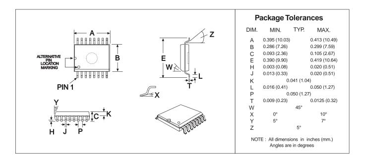
Figure 14: 16-pin SOIC Mechanical Outline: Order as part no. MX614DW
