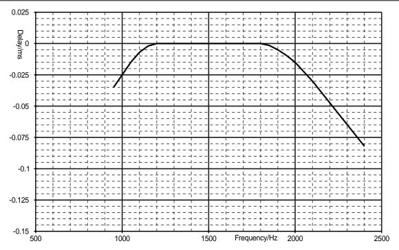
Figure 3: Rx Equalizer Group Delay (RXEQ = '1') wrt 1700Hz
