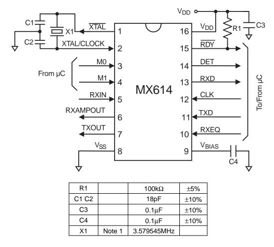
Figure 2: Recommended External Components for Typical Application
