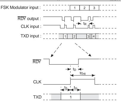
$t_D$  = Internal MX614 delay,  $t_R = \overline{RDY}$  low to CLK going low,  $t_S$  = data set up time  $tc_{HI}$ = CLK high time,  $t_{H}$  = data hold time
