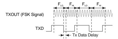
Note: M0 and M1 are preset and stable.  $F_{LO}$  and  $F_{HI}$  are the two FSK signaling frequencies.
