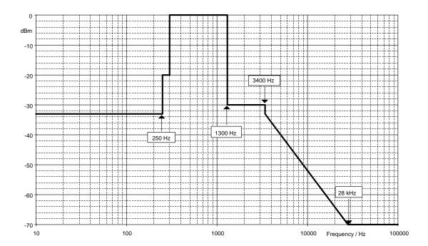
Figure 5: Tx limits at 5bps and 150bps rate
