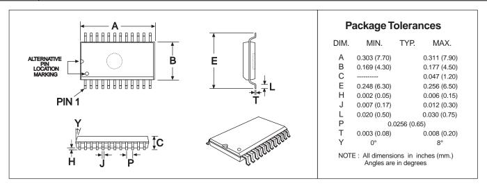
Figure 16: 24-pin TSSOP Mechanical Outline: Order as part no. MX614TN
