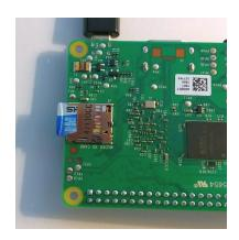
Figure 4: SD Card Installed in Pi
