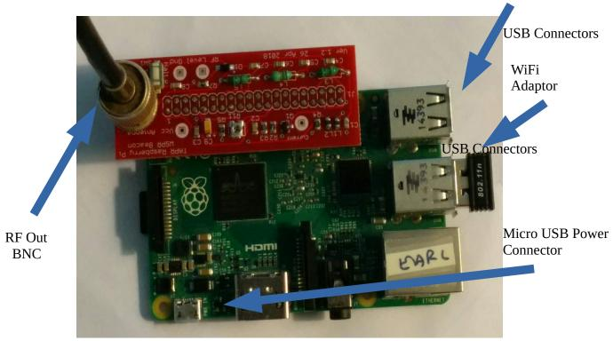
Figure 5: VW and Pi Assembly
