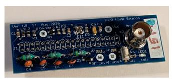
Figure 1: VW Board After Component Installation
