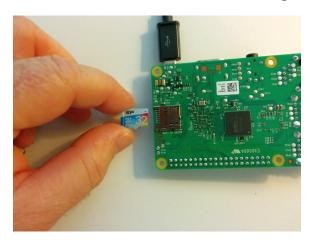
*Figure 3: Inserting SD Card into Pi*
