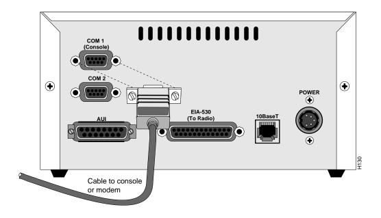
Service Console or Modem Connection to Router
