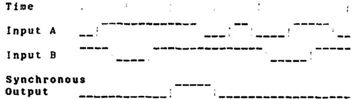
Looks a bit different, doesn't it? It turns out that we have to sample things faster than the changes at the inputs occur if we want to be able to approximate the old, non-synchronous output. It turns out that the sampling clock has to run at least twice as fast as the fastest event if we are to be certain of capturing every event.
