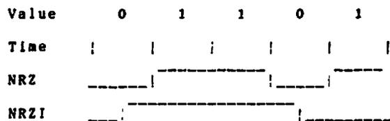
Notice that the value is determined in the middle of each time period. Also notice how simple NRZ is, and how confusing NRZI appears at first glance!
