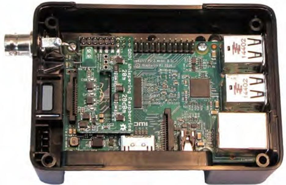
Figure 1. Raspberry Pi 2 with QRPI Shield installed on left.
