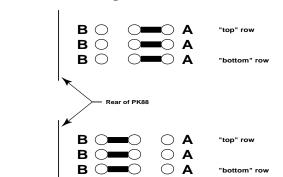
( ) On the bottom of the PK88 PC board add the following wire jumpers:
