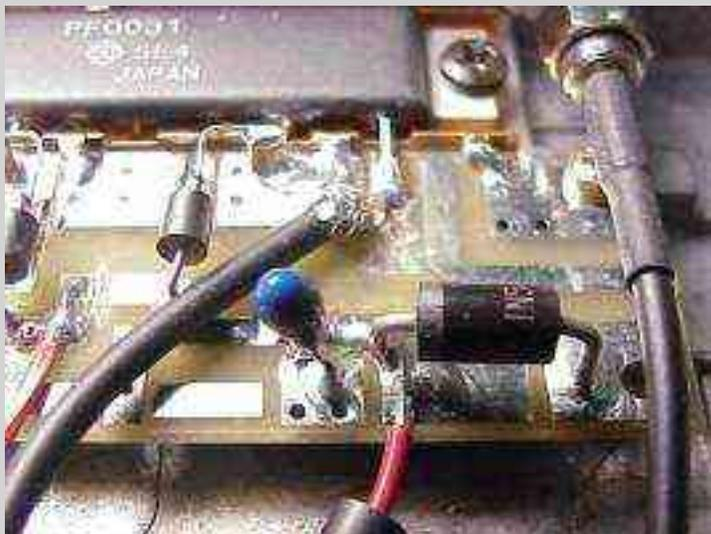
Closeup of the RF output side and the  $V_{dd}$  line. You can see the decoupling capacitors and the idiot diode.
