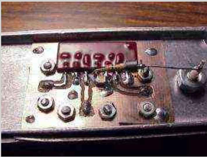
Closeup of the PIN diode module. You can see the bias resistor and ferrite bead floating in the air. The bias line passes through a regular feed-through (non-capacitor). RF connectors are SMA, with the teflon covered pin (ala the 33LNACK), the connectors are also available from [Down East Microwave](#).
