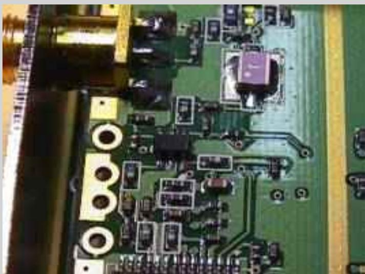
UPG152TA TX/RX switch and the bandpass filter.
