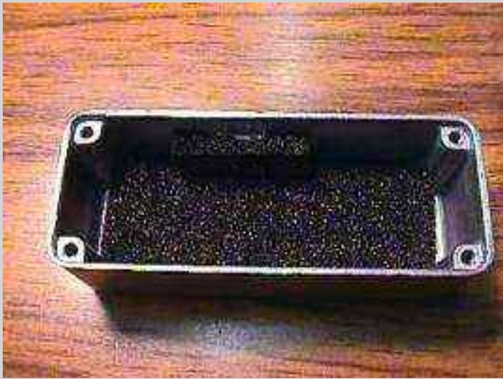
I lined the insides of *all* the cases with that anti-static foam you can buy at Radio Shack, part number 276-2400. Theoretically, this will absorb stray RF inside the case and help improve the circuit's input/output isolation. Or maybe I just smoke \$2 crack....
