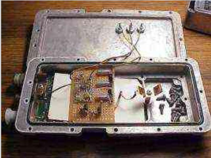
Picture of the transmit/receive control logic boards and the voltage regulators. Once again, housed in an old California Amplifier MMDS downconverter case. +15 VDC comes in through the top via a 1000 pF feed-through capacitor. The transmit/receive control logic from the WaveLAN card enters via one of the F connectors on the right side. The +5 VDC on transmit and +9 VDC on receive signals leave the case through standard feed-throughs (non-capacitor).
