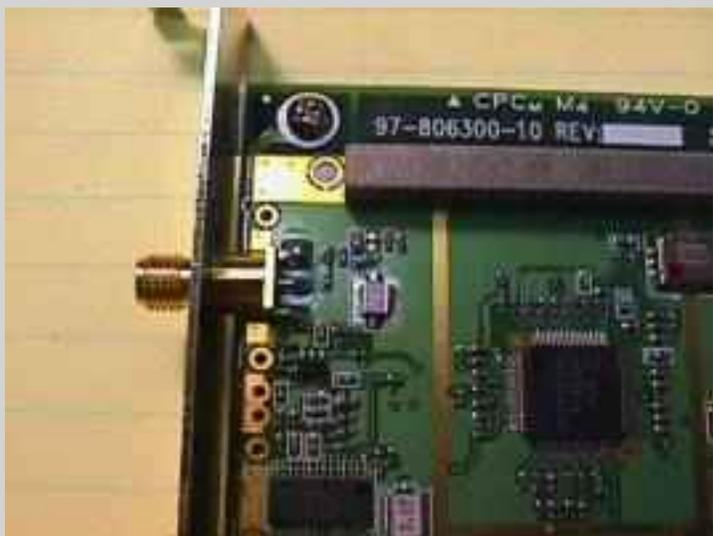
Antenna connector. Reverse polarity SMA connector. Diversity antenna switching is done by applying the DC control voltage via the coax to the included external diversity antenna.
