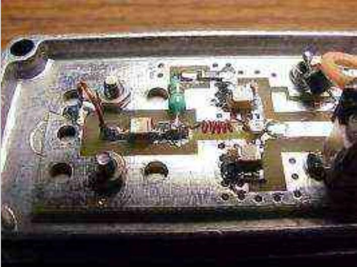
Closeup of the receive pre-amplifier's RF input, showing the shunt inductor and the modified series gate inductor.
