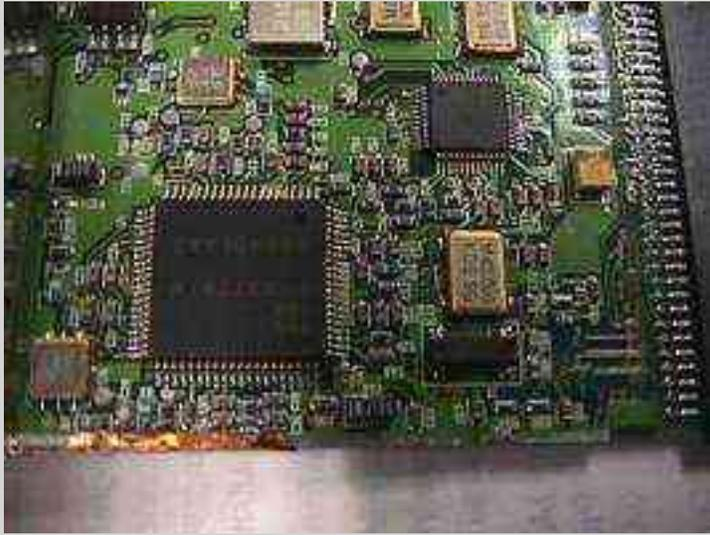
Shown are the HFA3726 400 MHz quadrature IF modulator/demodulator and the HFA3824 direct sequence spread spectrum baseband processor (small IC upper right) and their support components.
