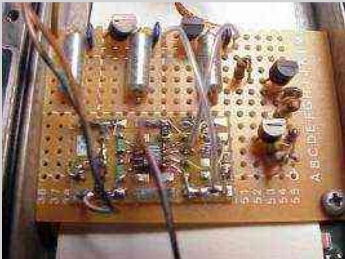
The 78L05 is shown in the top left, 78L09 is top right. The HRF49093 MOSFET is mounted on a surface mount carrier called a Surfboard. I used surface mount parts in the transistor switching logic for simplicity. *Ignore those two transistors on the right hand side.*
