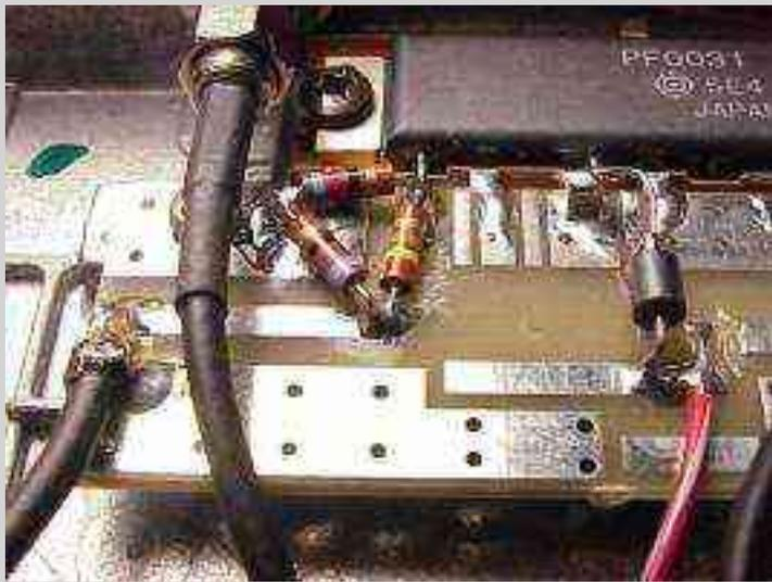
Closeup of the RF input side and the 20 dB attenuator. Should probably use surface mount resistors in the attenuator pad, but they won't handle the fairly high RF input power. You can also see how the circuit board was cut to isolate the  $V_{apc}$  line.
