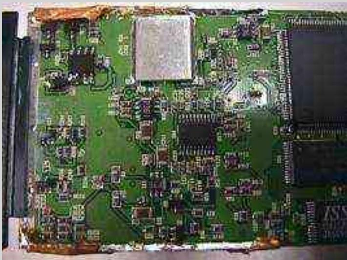
Shown are the HFA3524 dual frequency synthesizer and the associated oscillators and VCOs. Off to the right is the AM79C930 PCnet mobile wireless LAN MAC controller, the 128k flash RAM and the 32k SRAM.
