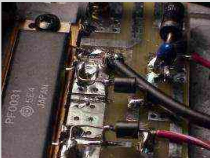
Alternate view to show how the  $V_{apc}$  and  $V_{dd}$  lines are supported in the air by the 56 pF ATC capacitors and the little jumper wires to connect them back to the rest of the circuit.
